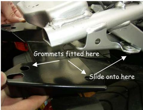
**Original spacers** The original fender bracket has a large slot the new Hamicad bracket has two holes but the fitting is as before using all the original fixings the only difference is that the spacer sits a little proud.
