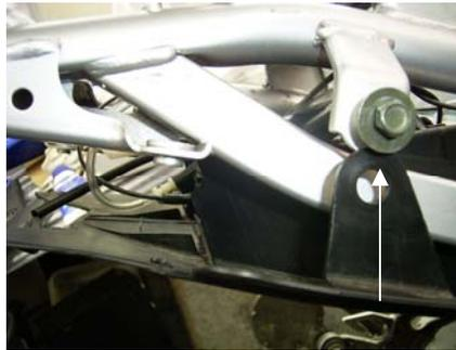
11 Remove bolts allow plastic tray to drop down( picture shows bolt replaced to prevent loss).
